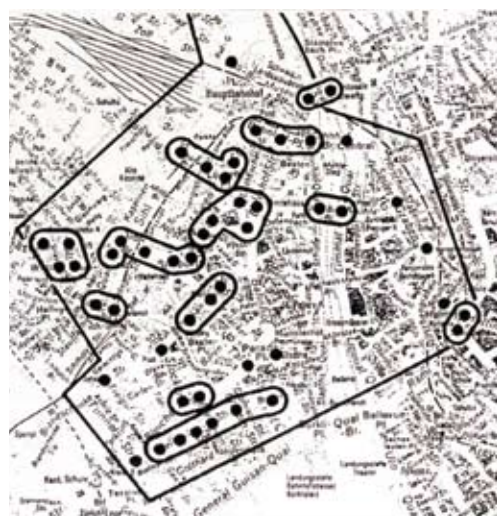
Figure 20: Zurich’s automobile traffic calming through traffic light cycle control: Traffic-calming is ensured by adapting the traffic lights system (a much shorter cycle favouring pedestrians, cyclists and public transport) Source: City of Zurich Police Department
